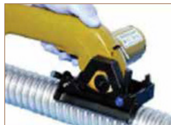
Using motorized saw to cut armor sheath to cut two adjacent convolutions on armor between 1.8 & 5 inches
