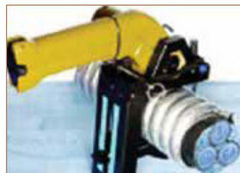
Motorized saw cuts armor and conductors
